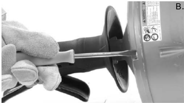
Figure 12 – Loosen 4 Drum Screws About 3 Full Turns, But Do Not Remove
